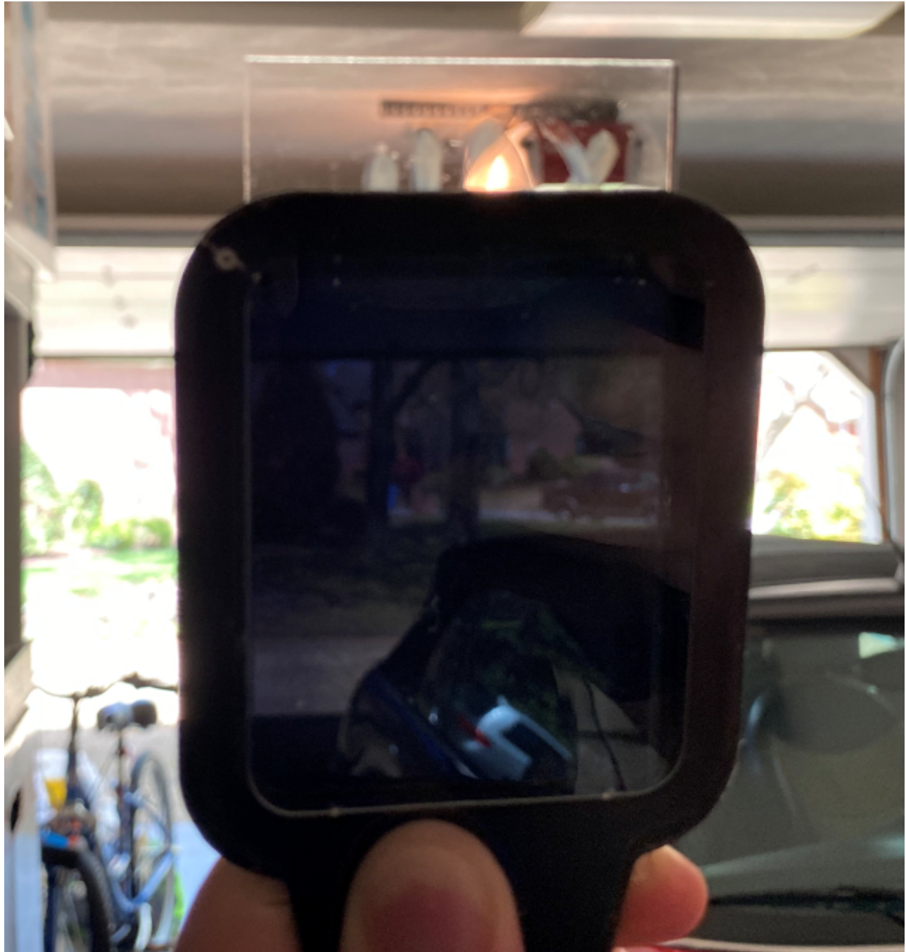
Figure 8: 24 Hour Radium-exposed plastic viewed through crossed polarizers
