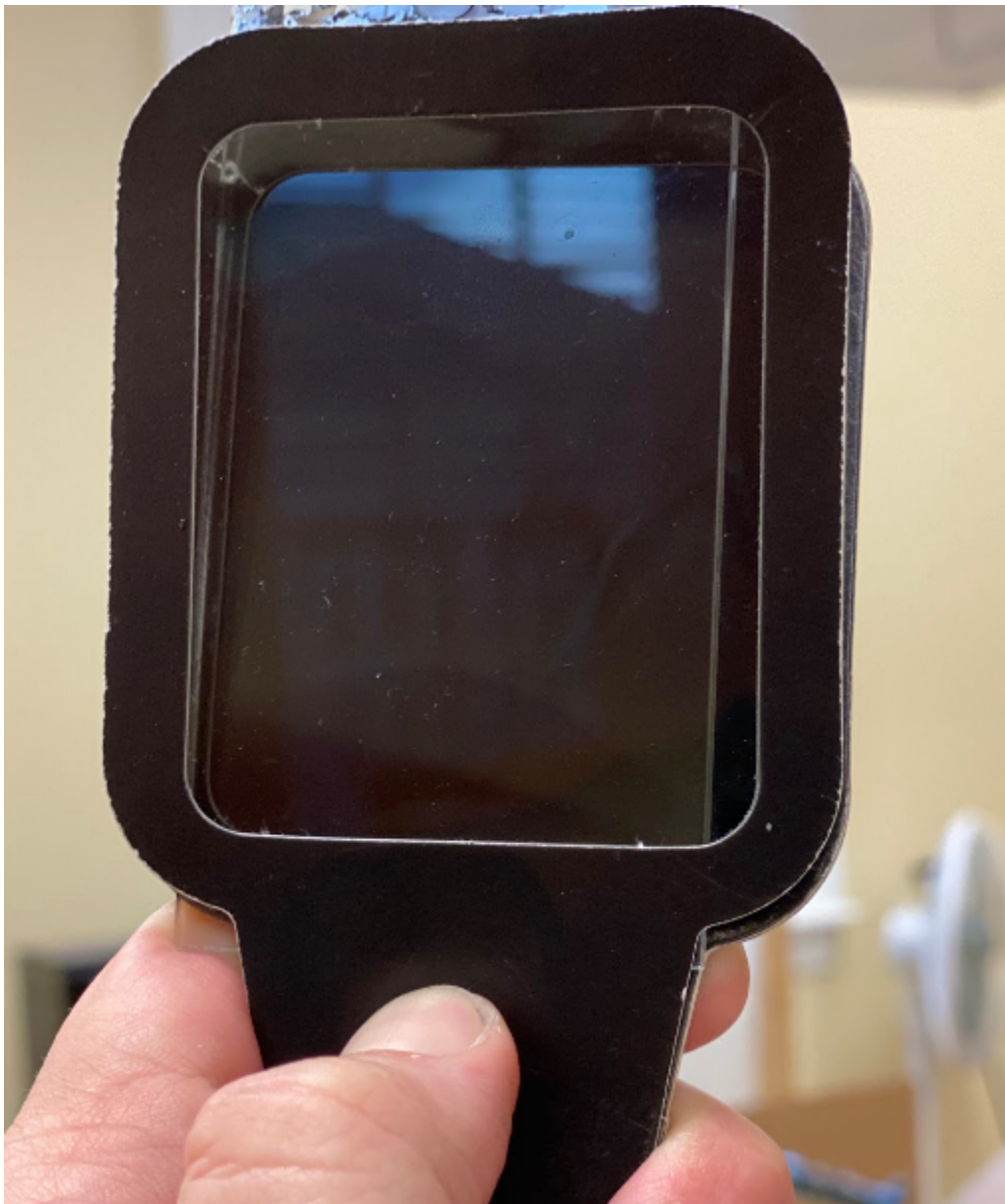
Figure 7: Unexposed plastic viewed through crossed polarizers
