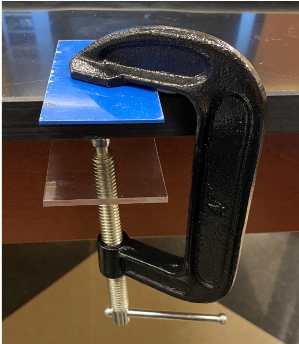
Figure 2: Bend Test Configuration
