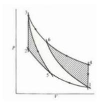
1-2-3-4 PV Process for Stirling/1-5-3-6 Process for Carnot
