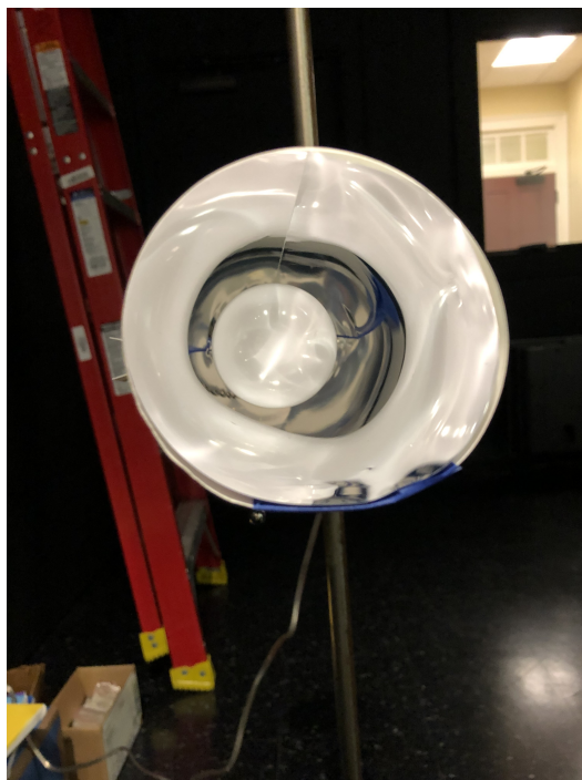
Figure 5: Light Tunnel with reflective mirror material
