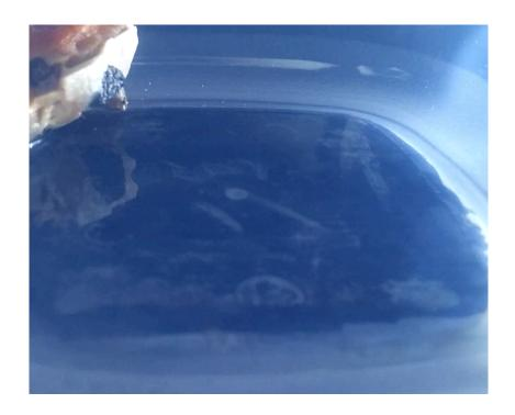
The reason for the increased visibility in the second photo is directly related to the temperature of the chamber. Here the chamber is running at -32C and the vapor trails tend to have a thicker more milky white hue.
