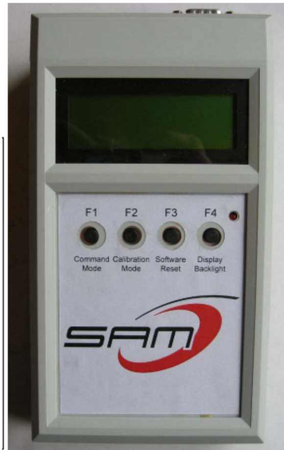
Figure 7: Enclosure Containing Keyboard, Controller, and Display PCB's [8]
