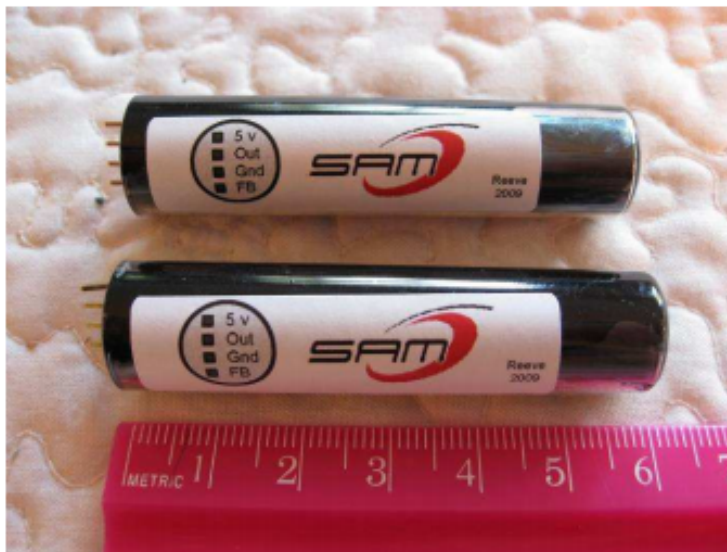
Figure 8: Two (of Three) Fluxgate Magnetometer Sensors [8]
