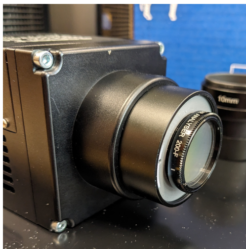
Figure 1: SA 200 attached to camera via adapter and 1.25" spacer
