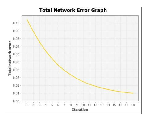
To enter data into the neural net, it first had to be normalized. Once this was done, the values could be given to the ANN and it would output a normalized value which then had to be unnormalized so that a comparison could be made. Below is the testing data for the neural net trained for range of motion in a vacuum.
