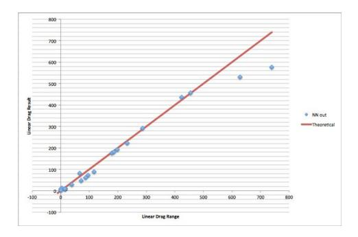
As seen in the graph above, the neural net did a good job of approximating the range for smaller velocities, but as the range of the projectile increased it became less accurate. This may have been due to a bias in the training data towards the lower values. The data was randomly generated in Excel, so it may not have been evenly distributed across the whole range.
