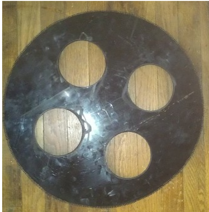
Photo of the 600 teeth wheel made from lexan
